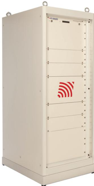
**ETS-Lindgren's Model 8100-126 RF Power Amplifier** is a 11000 W Pulsed Solid State power amplifier, designed primarily for EMC applications that include DO-160 and MIL-STD 464. Utilizing Silicon LDMOS technology, this RF amplifier provides higher linearity, rugged design in a more compact design.
