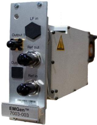
**ETS-Lindgren's EMGen™ RF Signal Generator Model 7003-003** is a modular signal generator with AM, FM, and pulse modulation, covering a frequency range of 4 kHz to 6 GHz. EMGen is designed for EMC testing, and quickly and accurately performs EMC tests without the need for an external modulation source. Using an internal modulator, EMGen provides CW, AM, FM, and pulse modulated signals.
