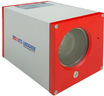
The **EMCam Camera Systems** provide color, high resolution images, making the systems an ideal addition for an EMC lab and monitoring DUTs. The cameras are shielded up to 200 V/m (CW) and 600 V/m (PM) with a resolution of up to 2 Megapixel. The SD Camera Cam5 offers an economical solution with lower resolution with manual zoom and focus.
