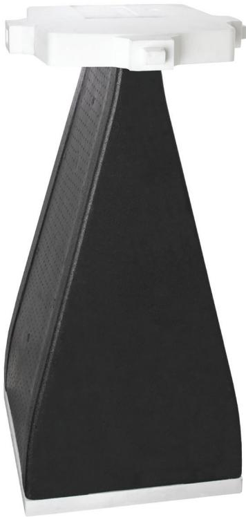
**ETS-Lindgren's DuraSorb™ DSH-1250H Absorber** is the latest evolution of ETS-Lindgren's, hybrid anechoic absorber technology. It combines the advantages of the proven FerroSorb™ performance with the physical properties of the PS Series absorbers. DuraSorb is constructed using substrates with rigid, closed cell foams that are loaded volumetrically and uniformly throughout the absorbers. DSH-1250H is ideal for 10m range chambers.
