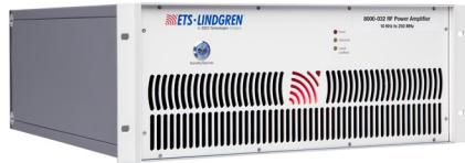
**ETS-Lindgren's Model 8000-032 RF Power Amplifier** is a 120W power amplifier, designed primarily for EMC applications that include IEC/EN 61000-4-6 requirements. Utilizing GaAs technology, this RF amplifier provides higher linearity, rugged design and better efficiency performance versus silicon-based amplifiers.
