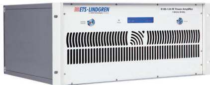
**ETS-Lindgren's Model 8100-124 RF Power Amplifier** is a 50W power amplifier, designed primarily for EMC applications that include MIL-STD 461 RS 103, 100 V/m requirements. This solid state RF amplifier provides higher linearity, rugged design and better efficiency performance versus silicon-based amplifiers.
