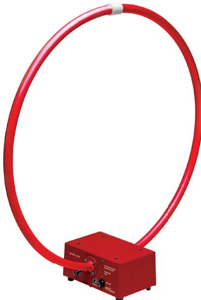
**ETS-Lindgren's Model 6502** is an active receiving loop antenna with a frequency range of 9 kHz to 30 MHz. This antenna is specifically designed to perform commercial emissions standards testing, such as CISPR 16-1-4. The Model 6502 can also be used for any magnetic testing, particularly MIL-STD-461B.
