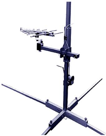
**ETS-Lindgren's Model 1052 Portable Antenna Tower** is useful for quick measurements, pre-scans, and anywhere a portable tower is needed. The model 1052 has two fiberglass mast sections, a hand winch, and four extending aluminum legs that are easily assembled/disassembled for ease of transportation.
